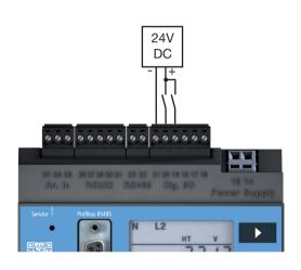
Fig. Connection example of digital inputs.
