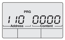
Fig. Display example; measurement switch for the baseline measurement, address 110 with a content of 0.
