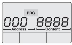
Fig. UMG 605-PRO display in programming mode
