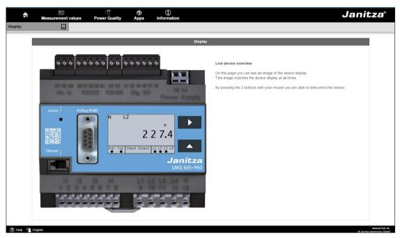
Fig. Operating the UMG 605-PRO via the device homepage
